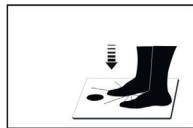
**AUTO STEP ON** – just step on the scale and stand still, the scale will automatically turn ON and start taking measurements.
