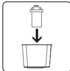
**4.** Insert the filter into the filter box so that it is securely in place. To do this, pull it down with a slight twisting motion and a little pressure.
